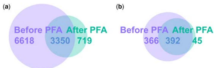
Figure 22 Euler diagrams describing the number of markers with intensities above 10,000 detected in: (a) positive ionization mode and (b) negative ionization mode by UPLC-IMS-QTOF analysis from WWTP discharge (Nov 6, 2018) before (purple) and after (green) disinfection with 2 ppm of PFA for 10 min, along with the number of common markers present in both samples before and after PFA addition. The areas are proportional to the number of markers in each zone.
